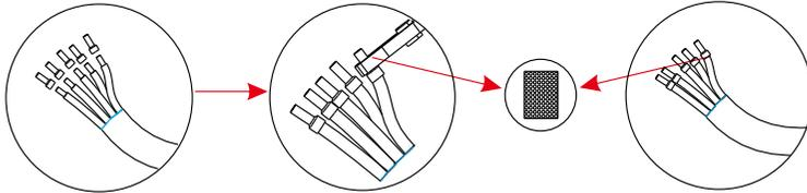
7. Insert the tripped end of each five wires into the appropriate hole in the female insert, and then tight each screw (to tight each wire in place).
