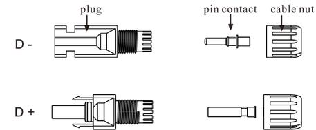
5. Insert stripped cable into pin contact and ensure all conductor strands are captured in the pin contact.
