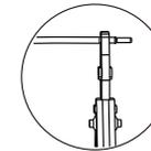
7. Insert pin contact through the cable nut to assemble into back of the male or female plug. When you feel or heard a "click" the pin contact assembly is seated
