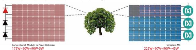
Seraphim MX reduces the shading effect significantly, prevents hot-spot formation, and eliminates diode failures. In the meantime, it will lower Operation and
