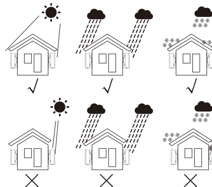
▲ Figure 4.1 Recommended Installation locations
