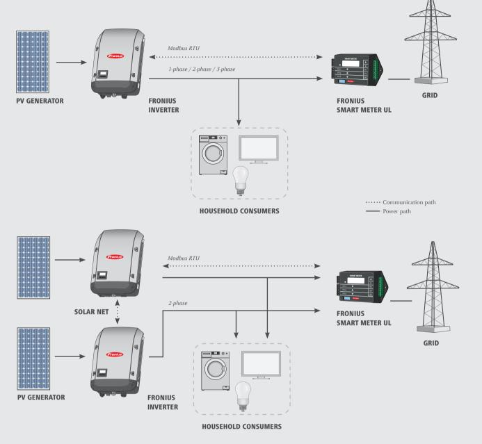
/ The Fronius Smart Meter UL works in conjunction with the Fronius Datamanager 2.0 via the RS485 interface (Modbus RTU) on the Fronius IG Plus inverters. The Fronius Smart Meter UL can be retrofitted at any time together with the Fronius Datamanager 2.0 on all Fronius inverters.
