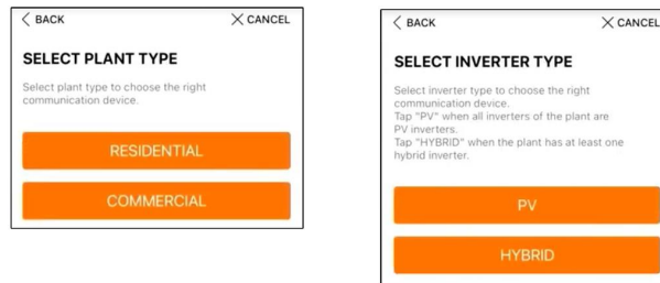
figure 6-3 Selecting Plant/Inverter Type
