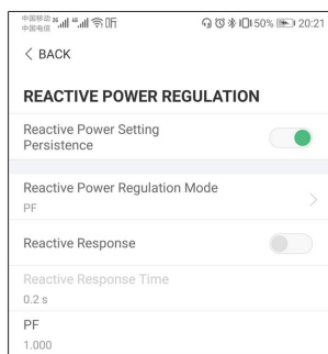
figure 7-17 Reactive Power Regulation
