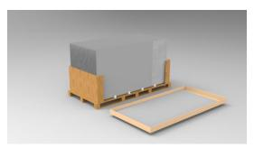
Use a minimum of four foam strands, placed evenly between the stacked modules.
