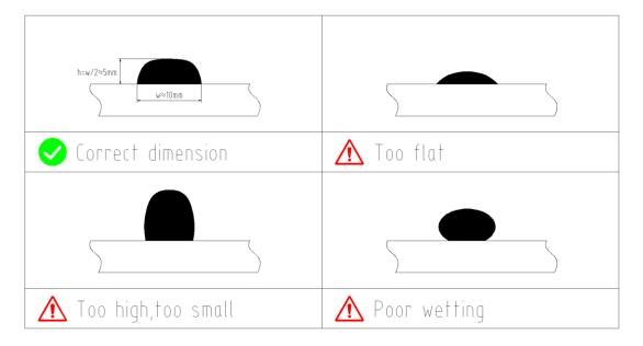
The correct form of structural adhesive after pasting modules
