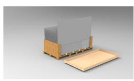
9. Place the box cover open side up and transport the module flat inside the cover to the project designated installation site Place a maximum of two modules in the cover, separated from each other with foam inside the box
