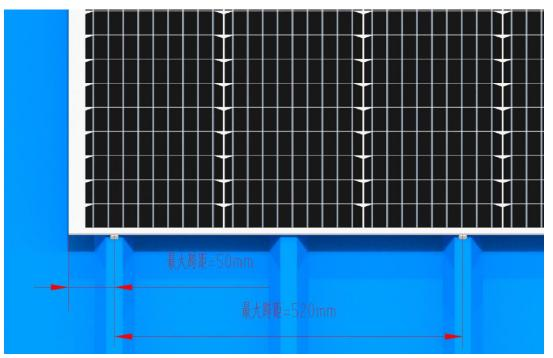
If there is a joint in the aluminum tube, the joint shall be placed between the modules.
