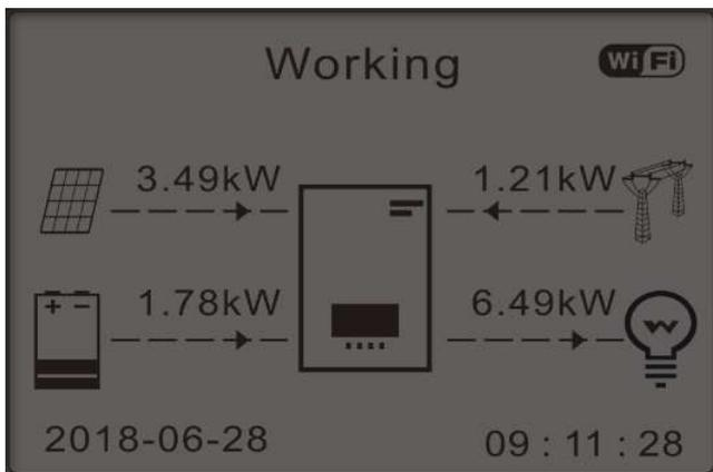
6) Press "DOWN" button to view current grid/battery parameters, press "UP" to get back to main interface.
