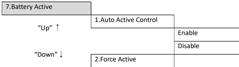
HYD-ES inverter can activate flat batteries when needed.
