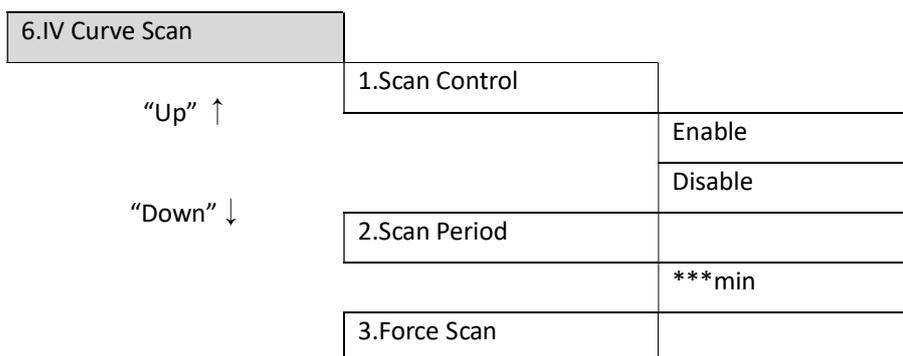
The user can enable “IV Curve Scan” (MPPT scan) to make HYD-ES inverter to find the global max power point periodically to deliver max power from a partially shaded PV array.
