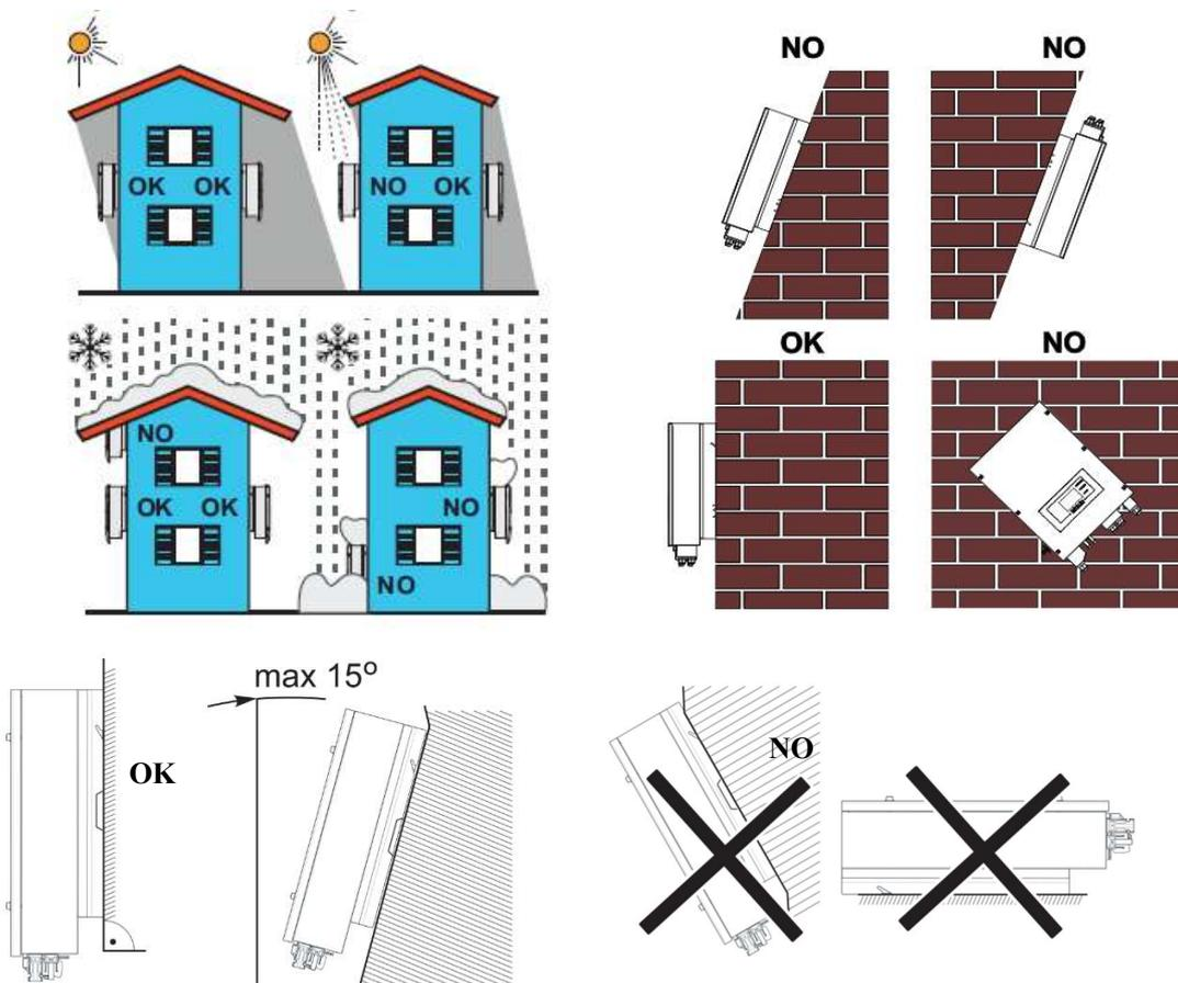
Fig. 4 Installation Position of HYD-ES inverter
