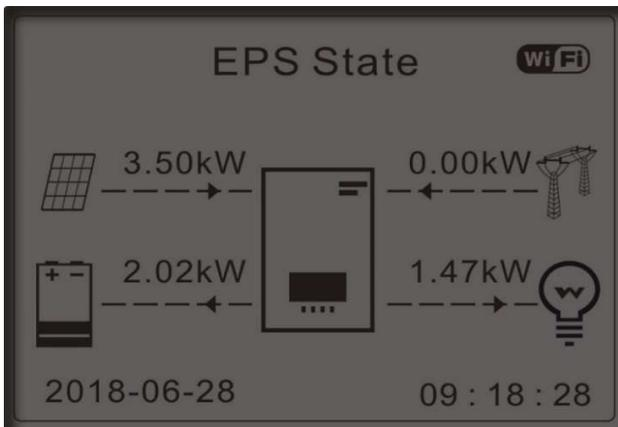
2) If PV generation = LOAD consumption, HYD-ES inverter won't charge or discharge battery.
