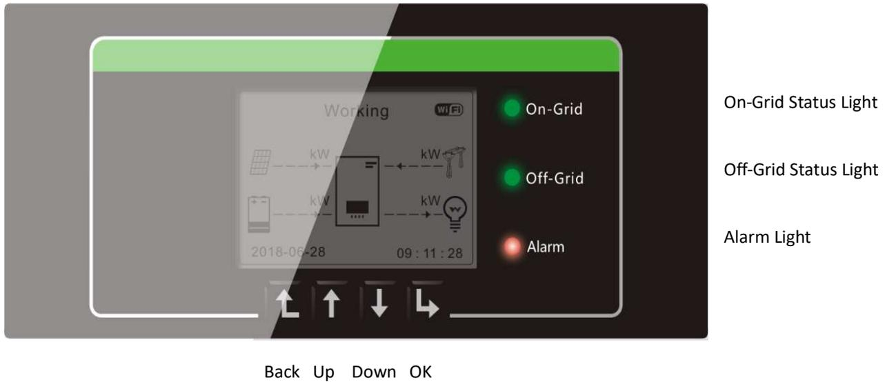
Fig 16. Buttons and indicator lights
