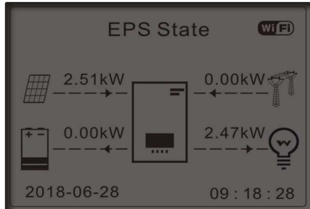
3) If PV generation < LOAD consumption ( $\Delta P > 100W$ ), HYD-ES inverter will discharge battery.
