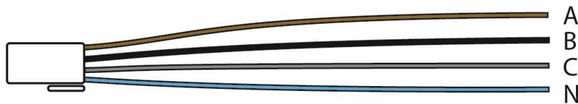
Figure 24: Voltage Line Harness for Three-Phase Service
