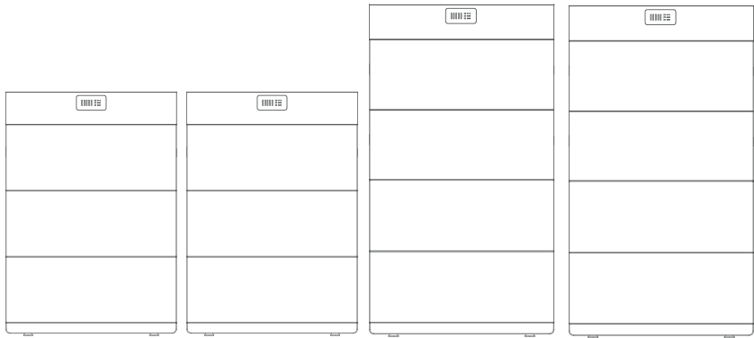
Two sets in parallel / three or four packs in series of each set
