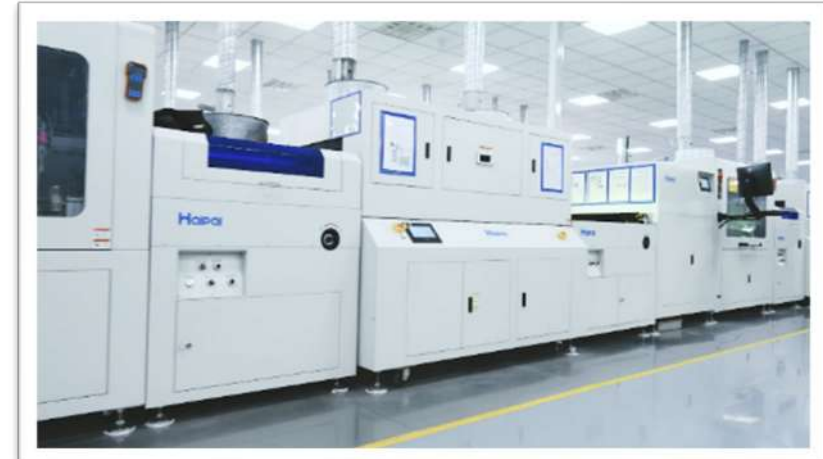
Three-proof Paint Spraying Workshop
