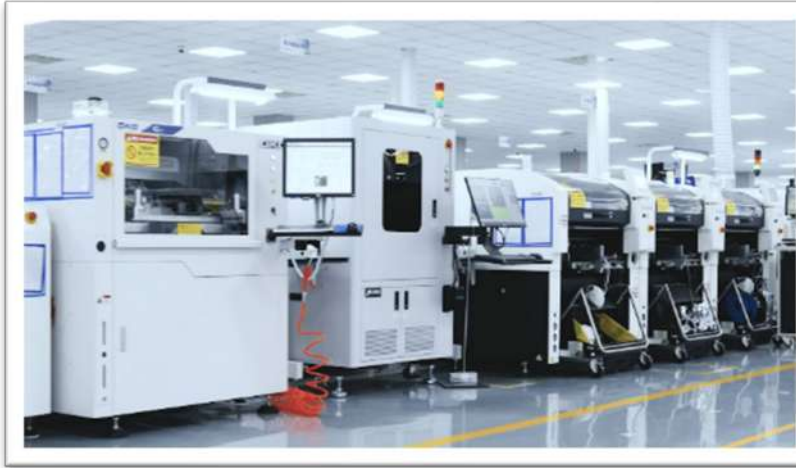
Ultra-high Speed SMT Mounting
